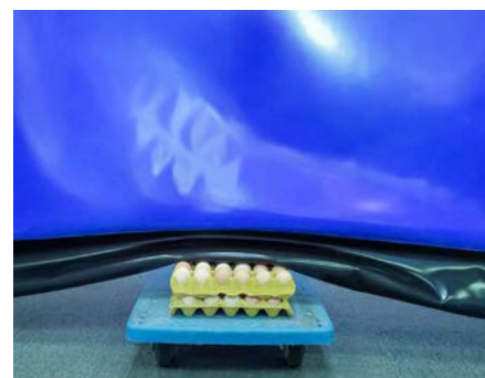
Safety bottom edge rebound system upon obstruction(Patented technology)
