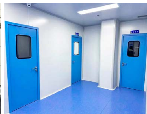
Steel Cleanroom Swing Door
